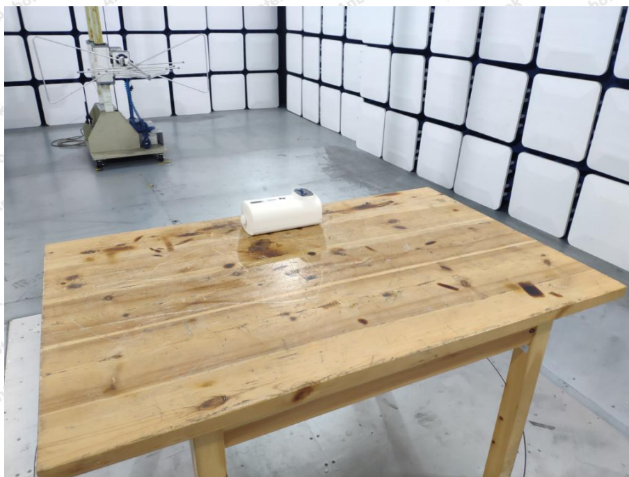
Photo of Radiated Emission Test
